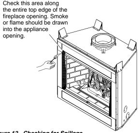
Figure 12 - Checking for Spillage
